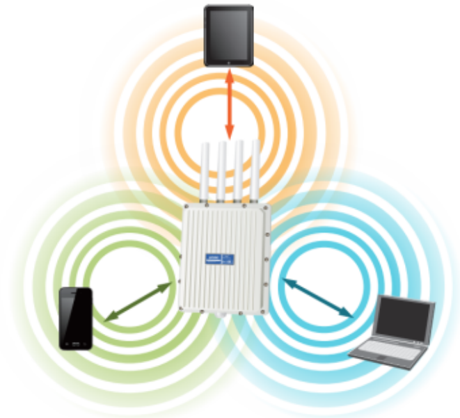
MU-MIMO Serving multiple users simultaneously
